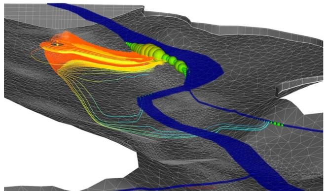
Visualisation of water sources (bullets), flow traces and travel times for a pumping well.
