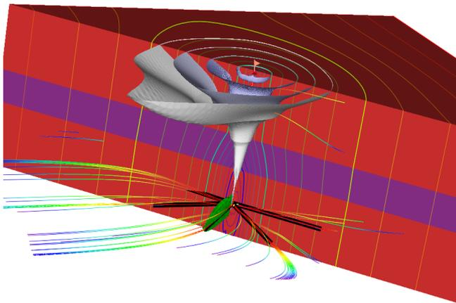
3D capture zone of a Ranney collector well (combination of vertical and horizontal well screens).
